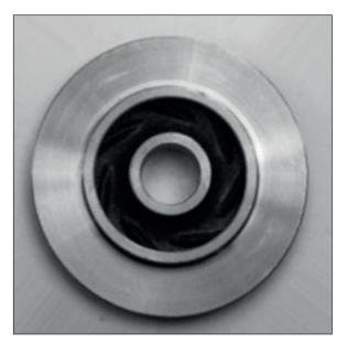
Fig. 9. Type II error - incorrectly classified rotor ",cast\_def\_0\_150.jpg". [31]
