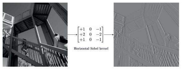
Fig. 3. Image transformation with Vertical Sobel kernel filter [29]
