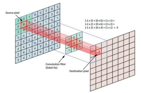
Fig. 2. Convolution filter - the idea of work [28]
